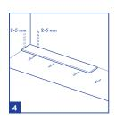
Make sure that you leave an expansion gap of minimum 2mm (0,08inch), preferably 5mm (0,20inch). For installations with floor heating, you need to leave an expansion gap of minimum 5mm (0,20inch). Never block the floor.
